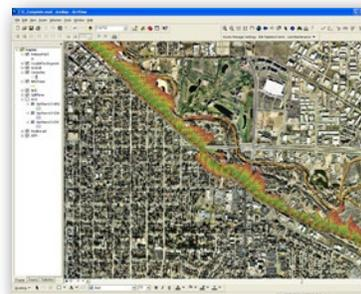
User specified release points are applied to demonstrate overland spread and water transport analysis for a hazardous liquid pipeline.
