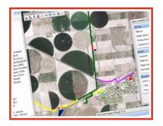
Gas HCA Analyst is a software application that determines how many structures fall within proximity of a pipeline (Class Location) and identifies high consequence areas (HCA) and regulated onshore gathering lines. Pipeline operators and engineering firms use this tool to quickly, accurately, and reliably run the analysis and prepare for submittal to meet DOT regulations.
