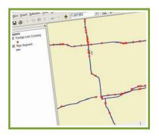
SpatialSynchronizer easily integrates PODS with Esri ArcSDE to illustrate changes in real-time. It uses the concept of dynamic segmentation to automatically place graphics at the correct geographic location based on stationing or chainage.
